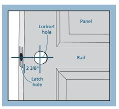
instructions and template, drill for lockset. Generally, a 2 1/8" diameter hole is needed for the lockset. Drill a 1" latch hole through the edge of the slab into the center of the lock hole to accommodate the latch for the lock. Some latches have a radius (rounded corners) or rectangular face plate that will require the slab edge to be chiseled for fit. Drill pilot holes for attachment screws. Other latches are round (contractor drive-in) and can be tapped into place with a
