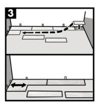
8. Start the third row with the plank cut at 1/3 of a length (16"). Again the remaining piece can be used at the opposite end of the row, if the layout of the room permits.
