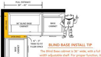
width adjustable shelf. For proper function, it must be installed a minimum of 3" away from the adjacent wall. This allows the doors to fully open and compensate for angle variances of the inside corner. In order to accommodate multiple width requirements, the Blind Base can be 'pulled' up to 9" away from the adjacent wall. This cabinet requires a minimum overall wall space of 39" in width to a maximum of 45" in width.
