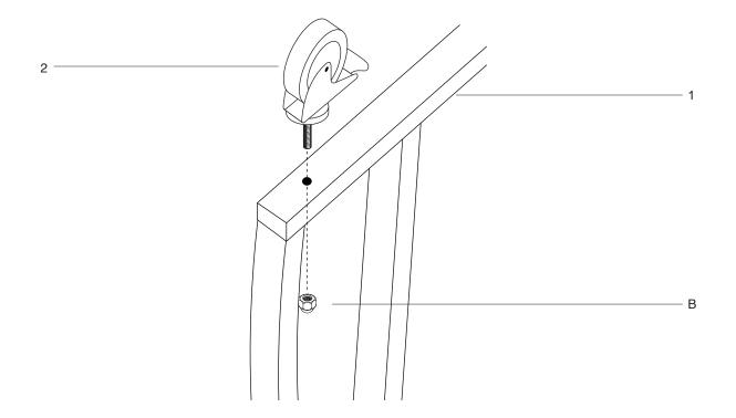
**STEP 1 -** Attach the four pre-threaded castor wheels (2 & 3) to each of the four brackets (1) by pushing them through the hole. Using an adjustable spanner secure each castor wheel with 1x nut (B).
