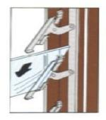
Install glass from inside by sliding in the clips . screen must be removed to install glass
