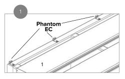
Secure Fiberon PhantomEC end clips a minimum of 1/4 in. from the wall with a single screw into the joist. Space clips no greater than 12 in. apart. Position the deck board into the end clip fasteners. It may be helpful to angle the board slightly to fully seat it into the clips.
