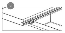
Insert a Fiberon PhantomGT fastener into the groove of the board, centering on joists.
