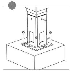
Determine the desired post locations. Use the base of the mount as a template to mark the four corner holes for the concrete Wedge-Bolt<sup>™</sup> anchors, included in the kit.
