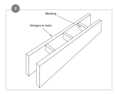
When installing blocking for more intricate decking patterns, remember that solid blocking (blocking laid on the flat) will inhibit water flow and result in buildup of organic materials over time, which will make cleaning more difficult. For best results when blocking is required, install ladder style.
