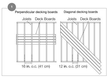
Joist location is important for the safety of the deck and will affect the layout, cost, and ease of installation for the railing system. If railing will be installed, determine rail post placment prior to joist construction. See page 9 for information about planning post placement for rail installations. Joists used in deck frame construction should be 2 in. x 8 in. (5 cm x 20 cm) or larger.
