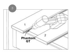
Secure GT fasteners by driving the screw fully into joist. Continue installing and securing the fasteners in the center of each joist along the remainder of the deck board.
