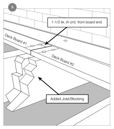
All brands of Fiberon decking may be surface fastened. Annular thread, ring shank and spiral shank nails, of sufficient length, have excellent holding power and produce good results, but screws have superior holding power. Use only screws designed for composite decking. Plain, galvanized surface fasteners are not recommended. Do not use traditional bugle-head screws.
