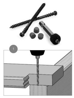
Locate all fastener holes at least 1 1/2 in. from board ends and 1 in. from board sides. For best results, pre-drill all holes with a 5/32 in. drill bit perpendicular to the deck surface to create the proper pilot hole and remove excess material to prevent cracking at fastener locations.
