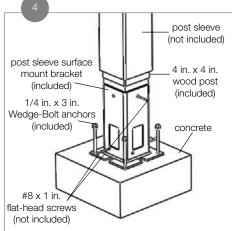
Locate the mount by aligning the mount corner holes over the drilled holes.
