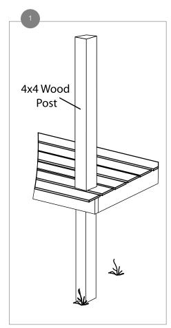
Ensure 4 in. x 4 in. (10 cm x 10 cm) wooden posts are code compliant and, where possible, spaced equally for the best looking application.
