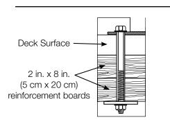
Note: The thickness of the wood/composite deck and reinforcement boards underneath the deck must be a minimum of 4 in. (two treated and structurally sound 2 in. x 8 in. lumber under the deck board), unless otherwise specified by local building codes.
