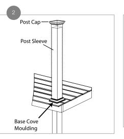
Determine the desired height of the post sleeve. Typically, the height is no less than 2 in. (5 cm) above the top of the finished railing system. This ensures the proper placement of the post caps that fit over the top of the post sleeve. Cut the post sleeve to the desired height.
