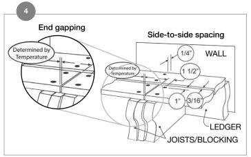
All decking materials, whether wood, composite or metal, undergo some degree of linear expansion with the changes of weather and the season. For best spacing results, keep boards out of direct sun during storage and cutting processes, and throughout installation if possible. Never cut and install boards in direct sunlight. To compensate for the effects of contraction and expansion, use short boards where possible with splitter/divider boards between each continuous run of boards.
