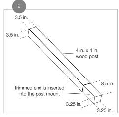
Cut the post sleeve to desired length.
