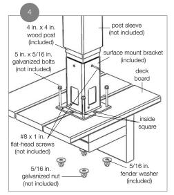
Insert the trimmed end of the 4 in. x 4 in. wood post into the mount. If necessary, place a shim under the mount to make the post plumb and true). If the wood post is loose within the mounting bracket, secure the wood post with (3)  $\#8 \times 1$  in. flat-head screws (not included) on the sides with prepunched holes.
