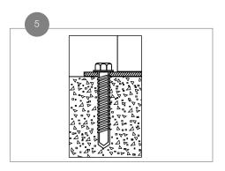
Fasten mount to concrete per local building code requirements. Insert the four concrete Wedge-Bolt anchors into the corner holes of the mount. Begin tightening the Wedge-Bolt anchor by rotating clock wise and applying pressure in toward the base. This will engage the first few threads as the Wedge-Bolt anchor begins to advance. Continue tightening until the head of the Wedge-Bolt anchor is firmly seated against the post mount. Repeat for the remaining fasteners.
