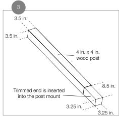
Cut the post sleeve to desired length.
