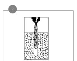
Drill the marked holes per the local building code requirements. Using a 1/4 in. masonry drill bit, drill the holes into the concrete base to a depth of at least 1/2 in. deeper than the length of the 1/4 in. x 3 in. Wedge-Bolt anchors. Blow the hole clean of dust and debris.
