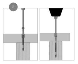
Using the Cortex setting tool, drive the fastener to the preset level below the deck surface in one continuous motion perpendicular to the deck surface. Install two fasteners at every joist and/or stair stringer. Overtightening will induce cracking at fastener locations.
