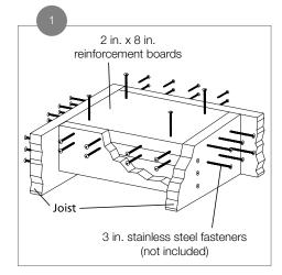
Determine the desired locations and fasten the reinforcement boards with 3 in. stainless steel fasteners as shown, prior to install the deck surface. Continue to step 2 after the deck surface is installed.
