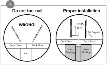
Always drive surface fasteners in at a 90° angle to the decking surface with two fasteners at every joist location. Do not toe-nail screws into the joist. Instead, place blocking/sister joists to allow perpendicular installation of surface fasteners at board ends.
