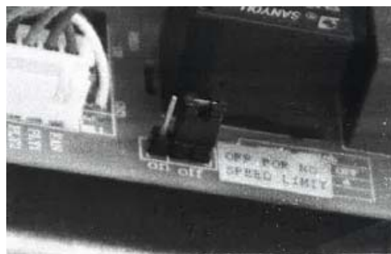
Speed limiting jumper shown in OFF position. Exhaust fan will now run at all speeds including Maximum.
