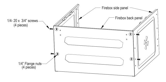
Assemble firebox front panel to firebox side panels using  $\frac{1}{4}$ -20 x 3/4 screws and  $\frac{1}{4}$ " flange nuts, as shown, tighten all screws. Again make sure to use the top and third hole down.
