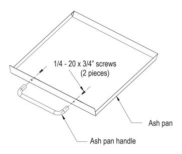
Insert the completed ash pan into slot underneath the main body of the grill.
