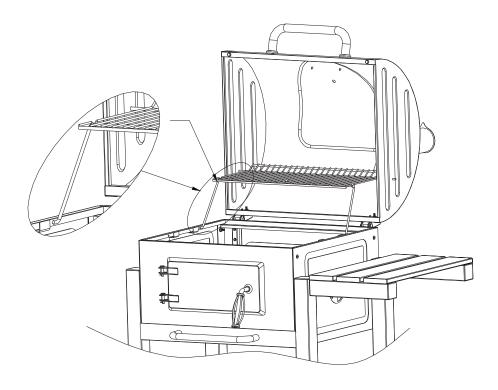
Attach 2 charcoal pan hangers to charcoal pan and place charcoal pan into grill. The charcoal pan hangers will hook onto the tabs on the inside of the grill.
