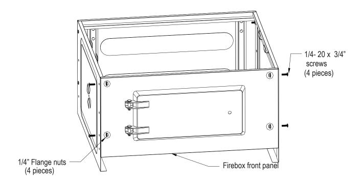
Assemble 2 left legs, 1 right rear leg and 1 right front leg to firebox and bottom shelf. Use four  $1/4-20 \times 2\frac{1}{2}$  "screws for the bottom shelf and eight  $1/4-20 \times 3/4$ " screws for firebox, tighten screws as shown in the figure.
