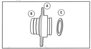
2. Screw hose barb assembly onto pump in clockwise rotation until hose barb assembly is tightened securely.
