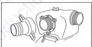
3. Slide hose clamp (A) over end of hose (B). Slide suction hose onto hose barb (C). Tighten hose clamp securely using a standard 1/4" (6mm) screwdriver.
