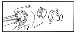
3. Slide hose clamp over end of discharge hose. Slide discharge hose onto hose barb. Tighten hose clamp securely using a standard 1/4" (6mm) screwdriver.
