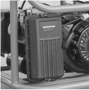
Figure 14 - Air Filter Casing.
