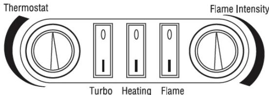
**FLAME:** Press this button into the "I" position for main power and flame effect. The indicator light will turn on.
