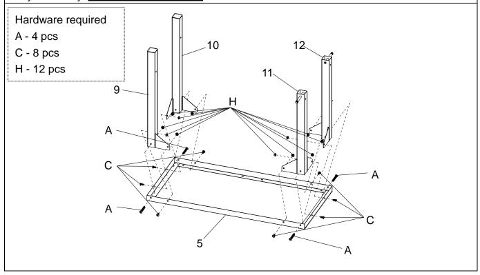
Step 2. Attach Storage Rack to cart assembly in previous step. <u>ONLY HAND TIGHTEN</u> bolts and nuts for now
