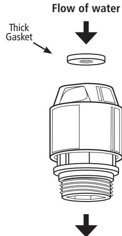
**Vacuum Breakers** are required by many municipal governments to protect the drinking water from being contaminated by water from swimming pools, lavatory sinks, bath tubs, or toilets. It is an atmospheric-type back flow preventer. The seating and unseating of the diaphragm are accomplished by the presence or absence of water pressure, when the unit is open to the atmosphere.
