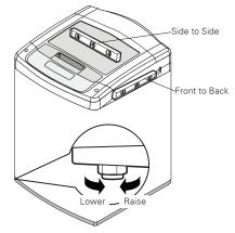
• If the leveling feet have been adjusted as much as possible and the washer is still not level, use the risers to lift the back leg(s) of the washer to help level it. To use, press the riser onto the leg. You can stack up to three risers under one leg.
