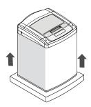
If you must lay the washer down to remove the base packaging materials, always protect the side of the washer and lay it carefully on its side. DO NOT lay the washer on its front or back.
