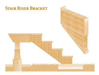
Stair Riser Brackets work in tandem to give strength and support while providing uniformity to your stair design. Easily bolted together, Stair Riser Brackets offer limited measuring to achieve maximum results.
