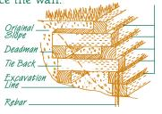
tie back and "deadman" will require more extensive excavation into the slope. These supporting timbers are leveled to lie on one course of wall timbers and are spiked into the timber below before setting the next course.
