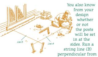
the house at that footing position. Example: for a 10' wide deck with l'overhang on each side, you would start your line 4' out from the midpoint of the ledger board.
