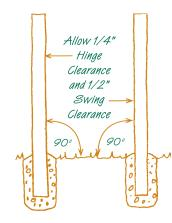
a gate, the first step comes when you are setting your face posts. Posts to either side of the gate should be absolutely plumb and set at least 24" in concrete.
