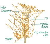
addition of a tie back with a stationary stabilization member known as a "deadman" to reinforce the wall.
