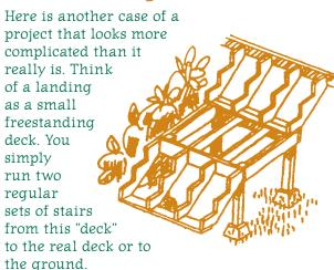
The most critical part of building stairs with a landing is the planning. You must first measure where you want the stairs to begin and end; then you can build the landing at the proper height, and in the proper position in relation to the deck
