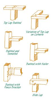
Rails are most easily set with galvanized metal\* fence brackets and nails. They may also be butted and toenailed, lapped, blocked or set with a dado. In each case, be sure to use galvanized\* nails. Drill pilot holes and stagger the nails in your rails to avoid splitting along grain lines. Attach the fence boards according to the style you have selected. Using
