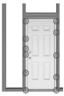
From the outside and with the door closed, ensure that the frame is in a straight vertical plane (not twisted). To do this check that the weather-stripping on the latch side is evenly compressed along the entire height of the door slab without any pinching or gaps.
