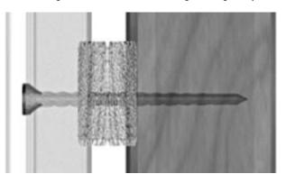
When the shims are properly installed, the frame should not move or twist at all when the screws are tightened and counter-sunk thereby maintaining the 1/8"gap. If there is any movement, loosen the screws and shim tighter to maintain the 1/8"gap, and then re-tighten the screws.
