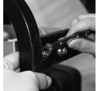
3.1 Lift the generator so that the alternator plastic cover is facing upward. Unscrew the ground terminal to release the ground cable using two 7/16" wrenches.
