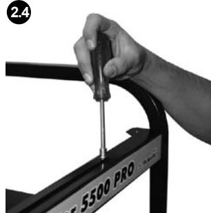
2.4 Unscrew the bolts using a 1/4" wrench from the tank heat deflector and then,
