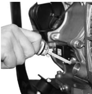
3.1 Lift the generator so that the alternator plastic cover is facing upward. Unscrew the ground terminal to release the ground cable using two 7/16" wrenches.
