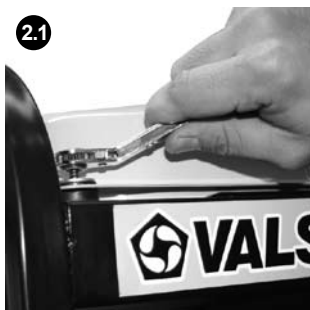
2.1. Use a 7/16" wrench to unscrew the 4 bolts
