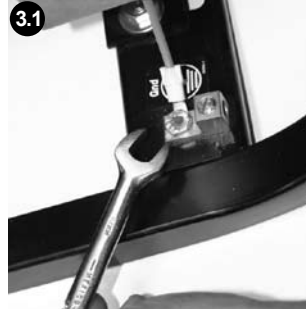
3.1 Lift the generator so that the alternator plastic cover is facing upward. Unscrew the ground terminal to release the ground cable using two 7/16" wrenches.
