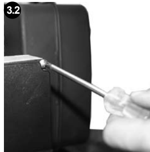
3.2 Remove the alternator plastic cover using a (Phillips) screwdriver.
