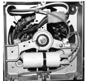
3.2 Remove the alternator plastic cover using a (Phillips) screwdriver.
