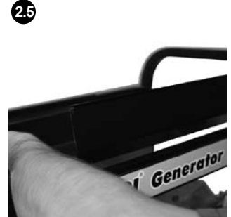
2.4 Unscrew the bolts using a 1/4" wrench from the tank heat deflector and then,
