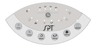
**ON/OFF button**: Turns the unit on or off Indicator light illuminates when unit is plugged in. Unit operates in default High fan speed.
