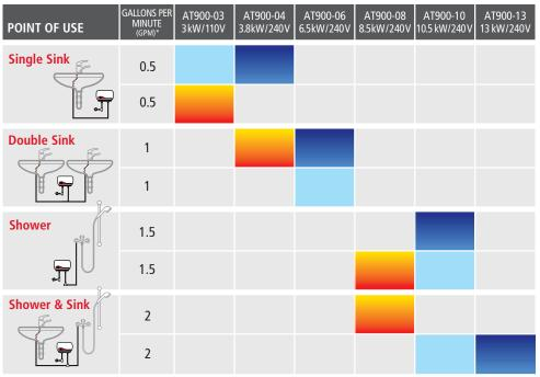
\* These values refer only to the hot water maximum flow rate at the device outlet.
