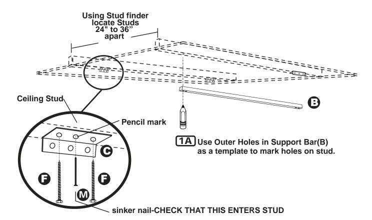
1B Attach Angles(C) into Ceiling Studs.
