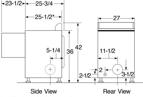
\*24-1/2" from the edge of the side panel to the front. 25-1/2" from front to edge of end caps.
