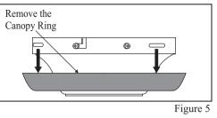
2. Remove the mounting bracket from the canopy by loosening the four screws on the top of the canopy. Remove the two non-slotted screws and loosen the slotted screws (Figure 6).
