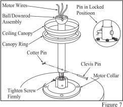
Align the holes at the bottom of the downrod with the holes in the coupling on top of the motor housing (Figure 7). Carefully insert the clevis pin through the holes in the collar and downrod. Be careful not to jam the clevis pin against the wiring inside the downrod. Insert the cotter pin through the hole near the end of the clevis pin until it snaps into its locked position, as noted in the circle inset of Fig. 7.
