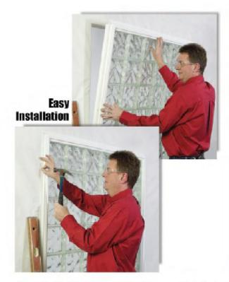
CrystaLok® Glass Block Windows are installed from the outside. Set the window into the opening with the weep gates at the bottom, use shims to assure that it is plumb and level, nail into place. Apply sealants, vapor barrier and flashing tape as you would with any new construction window.
