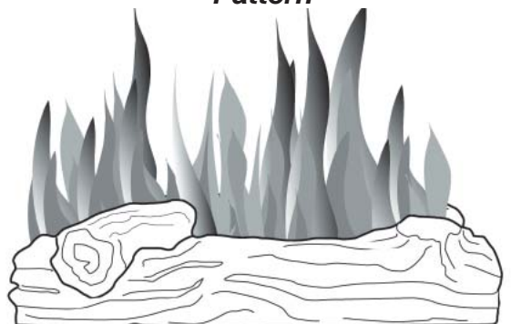
Figure 24 - Incorrect Burner Flame Pattern When Using Wrong Gas Type
