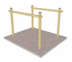
Lift, position and attach the second Post/End Girder section to post hardware.
