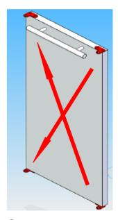
⑥ Move the "L" shaped door hinges of the upper and lower parts of the door to the left.
