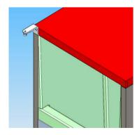
7 Turn the separated upper panel inside out and put it on the upper hinge and upper cover hinge bracket.
