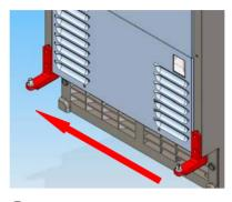
② Remove the anchor screws on the lower hinge and insert the hinge into the hole on the left.
