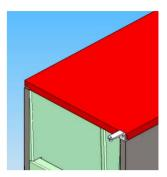
③ Loosen the anchor screws on the upper hinge and upper cover hinge bracket and remove the upper panel.
