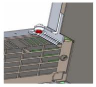
① Loosen the anchor screws on the lower hinge of the door and remove the door.
