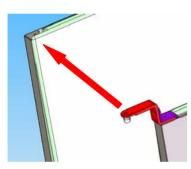
4 Remove the anchor screws on the upper hinge bracket and place the hinge into the hole on the left.
