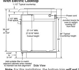
Note: For this installation, the bottom trim will not be flush with a typical 4" toe kick.
