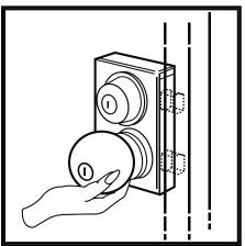
Align the lock holes in the locking jamb with the extended lock bolts, making sure the jamb is plumb. Mark, drill and fasten the locking jamb to the house using the one-way screws provided.
