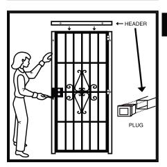
Insert plastic plugs into the ends of the header as shown. Mount the header jamb at the top of the door using the one-way screws provided. Leave approximately 1/8" space between the header and the top of the door frame.
