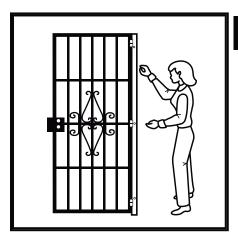
Position security door in front of opening at desired height, making certain that the security doors is plumb. Mark the location of the mounting holes in the door jamb, remove the door and drill 3/16" holes where marked. Replace the door, fasten the door to the house using the one-way screws provided.
