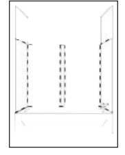
**11. CAULKING** Follow the instructions on the caulking tube and apply a bead of caulk along the bottom and top edge of the back and side walls. Also apply caulk to all vertical seams and edges.
