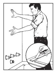
**10.** Remove the backing from the pressure sensitive tape. Place the appropriate panel edge carefully into the corner seam and press entire panel firmly to the wall. Move hand pressure up and down and side-to-side. Make sure all areas are in solid contact with the wall. Repeat the above for the opposite panel.
