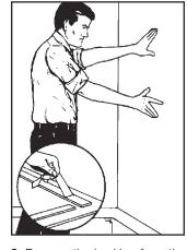
2. Remove the backing from the pressure sensitive tape. Grasp panel by the edges, carefully position to the right or left side of the back wall. Place panel edge into the corner and press firmly into place. Move hand pressure up and down and side-to-side, making sure all areas make firm contact to the wall. Repeat the above for the other panel installation.
