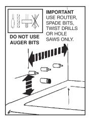
6. If the end of the tub has settled or the walls are out of plumb, it may be necessary to cut the bottom edge of a side panel(s) to achieve a level edge across the top from the adjoining back panel(s). Measure location of the plumbing outlets from the back wall forward and from the top tub ledge upward. Transfer these measurements to the side panel.
