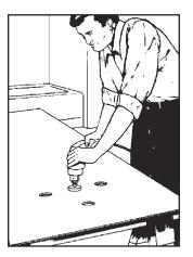
7. Cut holes 1/2" larger than the diameter of the pipes. Drill from the finished side of the panel. For best results place a scrap of wood beneath the hole to be made. This will ensure a clean cut.
