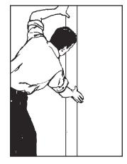
5. Carefully center the batten trim strip over the back wall panels (align your center marks) and press firmly into place from top to bottom making sure all areas are in solid contact with the wall panels.
