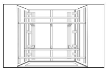
**12.** Trial fit the placement of the corner moldings and transfer the height measurement of the vertical seam to the corner molding. Trim corner moldings. Apply a 3/16" bead of adhesive in each corner seam. Press the corner moldings firmly into their appropriate corners. Immediately remove any excess adhesive with a damp cloth. Temporarily secure corner moldings to the back and side walls with masking tape. Allow adhesive to cure overnight.
