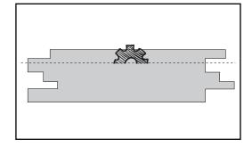
When you get to the top and final row you may find that you need to trim the overall height of the panel. This is the case if the height of the wall/surface doesn't equally divide by the height of each panel.
