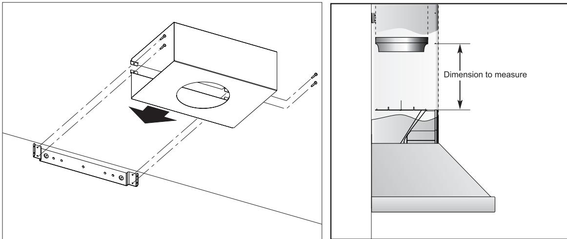
Cut the duct at the measured size.
