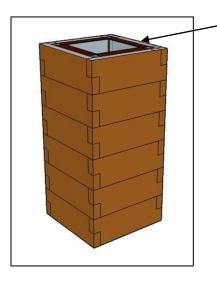
When you get to the top course, bend the flashing over the frame and screw in place.
