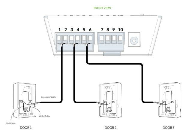
$IMPORTANT: When connecting \ Gogogate\ 2\ to\ wall\ console\ polarity\ does\ not\ matter.$
