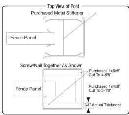
Post Spacing will be determined by gate width and hardware.
