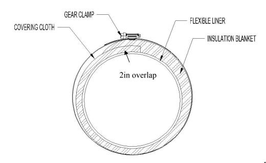
3. Next, install Lock N Go Tee Base onto liner. Insert liner into top of tee and snug up on gear clamp around liner. The branch will be installed later. Note: "IF" Insulation Blanket is used - Peel back the insulation in order to make a direct connection between the gear clamp of the fitting to the liner, then re-cover.
