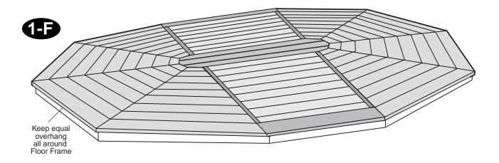
**1-G:** Removal of Center Panels may be necessary for easier assembly. Triangular Floor Panels are attached by using eight 2-1/2" screws only. Add additional screws where holes are predrilled for 12' and 14' floor. Predrilled holes are provided in each Floor Panel.
