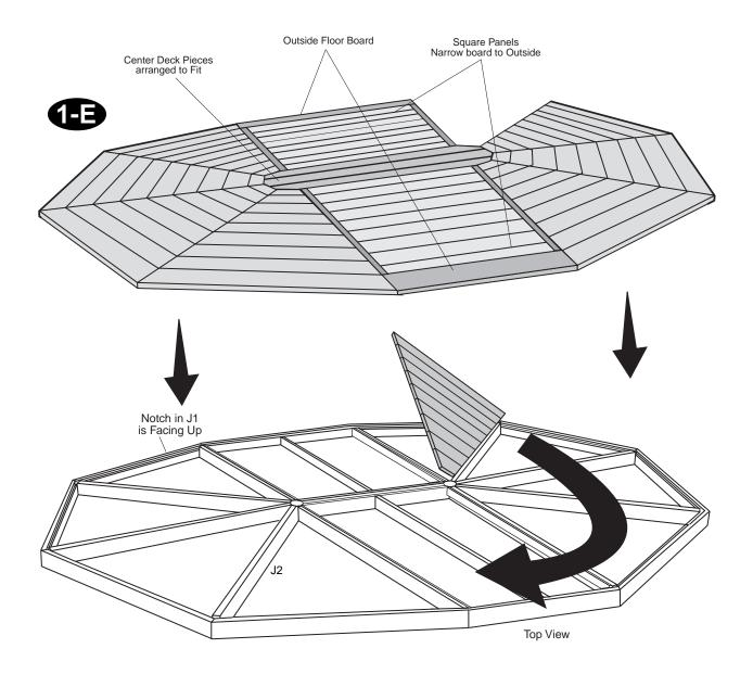
1-E: Carefully set Floor Panels in place. Align Floor Panels so that they are tight and equally spaced before fastening in place. Seams on Floor Panels should line up directly over center of J2's.
