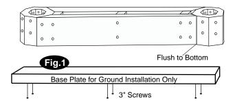
1-A: 14' Gazebo - Layout Center Floor Support (angled) and Center Spacers equally as shown. Use (2) 3" screws as shown. Install Hollow Center Blocks J3 as shown with 3" Screws. Note: If you are installing your Floor Kit above ground or on a soft surface such as grass, sand and loose pebbles, add Base Plate to Center Assembly as shown in Fig.1 with (6) 3" screws. DO NOT Use Base Plate on hard surfaces such as concrete or an existing wood deck.
