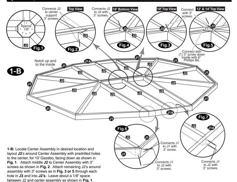
Layout all J1 and J1A parts on edge as shown, make sure that the notch on J1 is facing up and to the inside. Connect J1's and J1A's as shown in Fig. 6&7 with 3" screws. Keep joints even on top and outside edges. Assemble all in the same manner.
