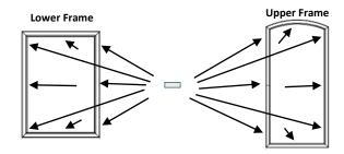
3. Remove one side of the paper backing from the double sided adhesive tab and firmly affix the tabs to the lower and upper frames in the areas shown above. The tabs must be adhered to the flat surface which is the approximate size of the tab. (Note: There are 16 tab adhesion points, 4 extra tabs are provided for your convenience.)
