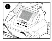
Locate and unlock filter cover as shown. Push left to un-lock, right to lock.
