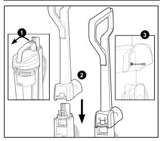
Remove the dust cup before installing handle.
