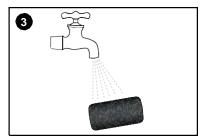
Wash with water every 3 months, allow at least 24 hours to dry and make sure it is dry thoroughly before re-using.
