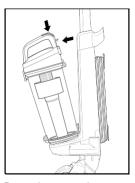
Press dust cup release button to remove the dust cup.
