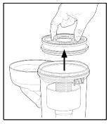
Remove the dust cup foam filter.
