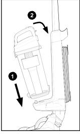
Place the dust cup back onto the machine and push until it clicks into place.
