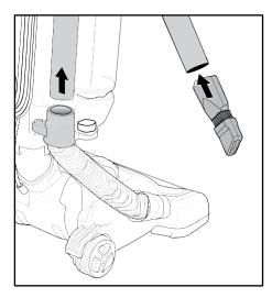
Remove hose handle and 2-in-1 crevice tool accessory from the machine.
