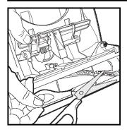
Carefully remove any string, hair or debris located on the brush roll.
