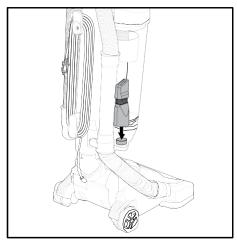
Insert the 2-in-1 crevice tool accessory into the on-board storage reservoir, as shown.
