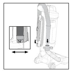
Insert the handle hose end into the conector hose and rotate clockwise to join. Then insert the handle into the other hose of the body.
