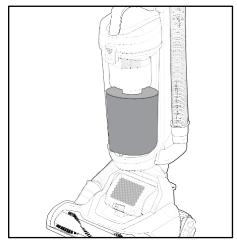
To maintain optimal performance, please emtpy dust cup when debris reaches MAX FILL line.
