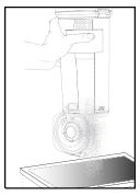
Close the base of the dust cup, align the cup base back onto the machine and push until it clicks back into place.
