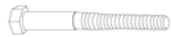
5/16" X 4" SS Lag Bolt (for connecting the 2" x 8" headers to the posts)
