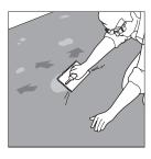
4. Areas unable to receive vertical flashing, such as pipe penetrations and bathroom tubs, should be sealed using a good quality silicone sealant. Run a continuous bead and tool the material to provide continuity to the membrane.
