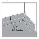
4. For inside corners, provide a relief cut, but place adhesive where the membrane folds over itself to ensure a waterdurable connection. Overlap butt joints by 1-1/2" and use the mastic to ensure a water-durable connection. Apply adhesive to the vertical and horizontal legs of the butt joint. Work the material carefully into position and smooth out, using the flat edge of the trowel.
