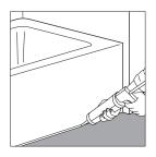
5. Allow membrane adhesive to cure sufficiently (minimum 2 hours for Durlock tile membrane adhesive, minimum 4 hours for Type 1 organic adhesive or 8 hours for latexmodified thin-set mortar).
