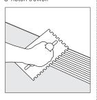
Install membrane with the cementitious side out. For outside corners, make a relief cut and press into adhesive. Use the trowel's smooth edge to fully embed the material.
