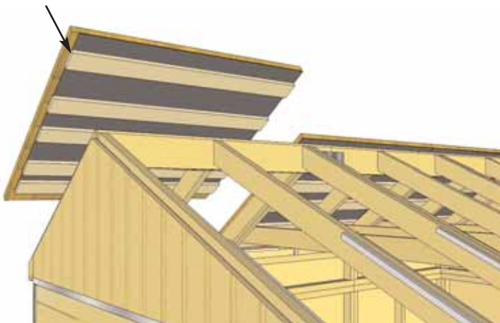
Shingles overhang battens on outside
