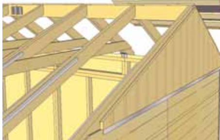
54. Identify all Roof Panels . There are 2 Outside Right, 2 Center and 2 Outside Left Roof Panels. The outside of the panels will have shingles overhanging the battens. Starting with an Outside Roof Panel on Short Roof Side, lift up and place a roof panel on rafters so centered on mid rafter. Lowest batten on roof should be flush with end of rafter at bottom.
