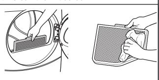
Clean the lint screen before each load. Pull the lint screen straight up. Roll lint off the screen with your fingers. Do not rinse or wash screen to remove lint. Wet lint is hard to remove. Push the lint screen firmly back into place.
