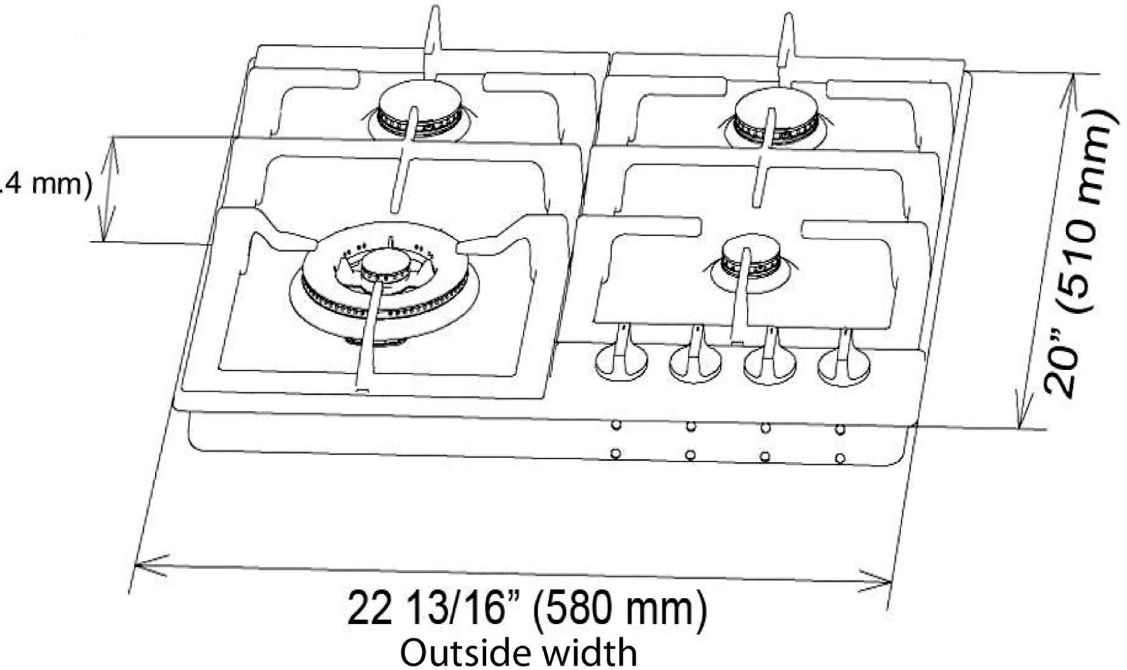
Required clearance from bottom of cooktop to top of built-in oven or cabinet.
