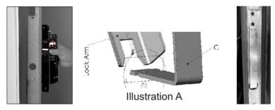
8. Now you will need to position the Lock-Bar-Hinge(D) inside the door track, by inserting the tabs of the Lock-Bar-Hinge(D) within the slots of the Lock-Bar(C).
