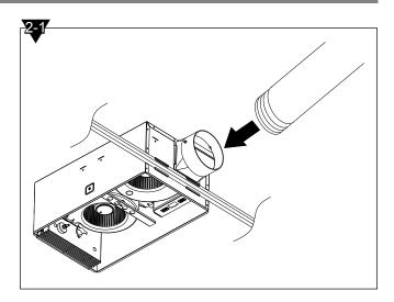
b. Do not install the unit where ducts are configured as shown in Figure 2-2. Install the duct with a gradient of 1°-2° to the outside.
