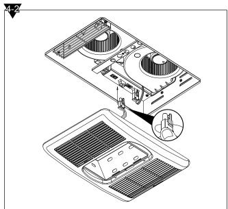
c. Install the Grille Assembly ② into the Fan Body ① using the Machine Screw ③.
