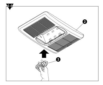
e. Install the Light Lens 4 into Grille Assembly 2.
