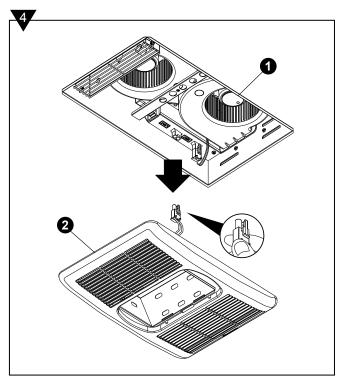
5. Remove dust and dirt from the Fan Body **①** with a vacuum cleaner.
