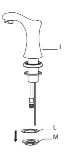
Remove mounting nut (M) and rubber washer (L) from spout (I)
