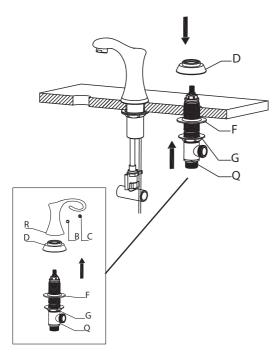
Remove cover button (C) from handle (R) and loosen set screw (B) with hex wrench (T). Remove handle (R), then remove base metal ring (D) from valve (Q). Insert valve (Q) into hole (Hot: Left, Cold: Right) from underneath. Repeat steps for second handle (A) and valve (H)
