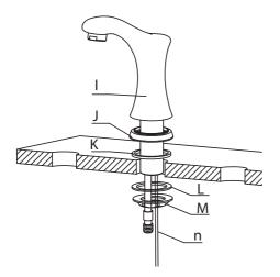
Install spout (I) through predrilled hole in sink or countertop with spout base (J), base O-ring (K), and lift pole rod (n) attached. Attach rubber washer (L), and mounting nut (M)
