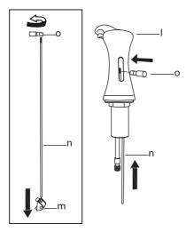
Remove lift pole knob (o) and clip (m) from lift pole rod (n). Insert lift pole rod (n), threads up, into the base of the spout (I). Place lift pole knob (o) in the back opening of the spout (I). Connect lift pole rod (n) to lift pole knob (o) and tighten
