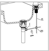
• Install clip (m) on lift pole rod (n) by pressing both ends of the metal sheet. Adjust clip (m) to the required height of the drain off pole (j). Insert drain off pole (j) into designated hole on clip (m)
