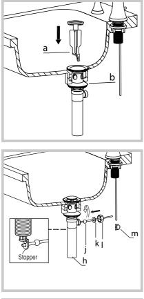
• Insert waste stopper (a) into drain (b). Make sure slot at end of the waste stopper (a) is facing the rear of the sink
