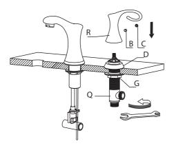
Connect base metal ring (D) onto valve from above. Tighten mounting nut (G) on valve (Q) from underneath with adjustable wrench until snug. Reinstall handle (R), tighten set screw (B), and insert cover button (C). Repeat steps for second handle (A) and valve (H)
