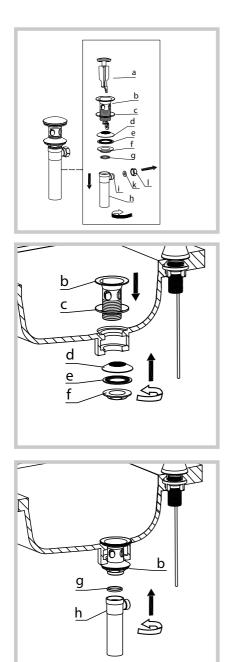
• Remove waste stopper (a) from drain (b). Remove tail pipe (i), mounting nut (f), plastic washer (e), and concave washer (d) from drain (b). Remove retaining nut (12) and washer (k) from tailpipe (h)
