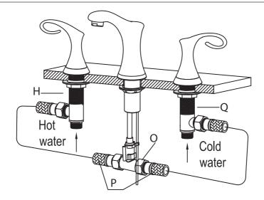
Thread waterlines (P) to hot and cold valve (H & Q) horizontally. Thread other end of waterlines to t-union (O). Attach hot & cold supply lines (not included with faucet) to valve (H & Q) vertically
