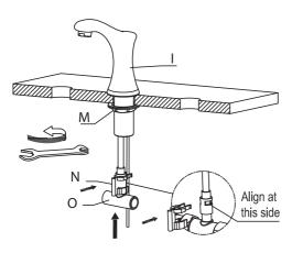
Adjust spout (I) to proper position and tighten mounting nut (M) with adjustable wrench. Install t-union (O) onto supply line of spout (I). Attach t-union clip (N) to secure t-union (O)
