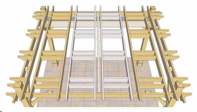
**9.** With Drive Beam and Canopy secured, attach Pergola Ladder Sections as per **Step 17** of Breeze Pergola Main Assembly Manual.
