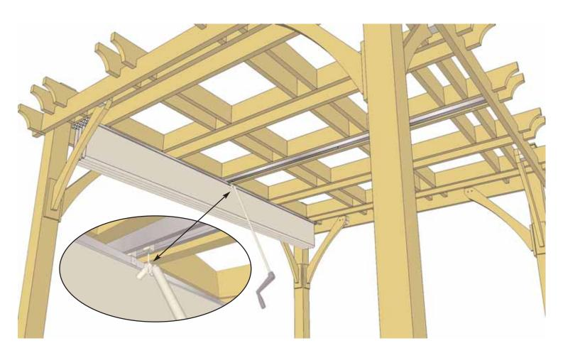
**10.** To retract the Canopy, locate the Canopy Pull Handle and place end into Locking I-Bolt. The Canopy can be locked and unlocked by turning the I-Bolt with the Pull Handle.
