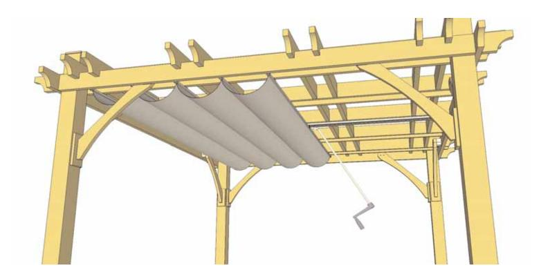
**11.** To retract the Canopy, unscrew locking I-Bolt with the Handle and pull the Canopy to desired length and lock. To close, follow same procedure. Be sure to place Canopy Pull Handle in safe and secure location for future use.
