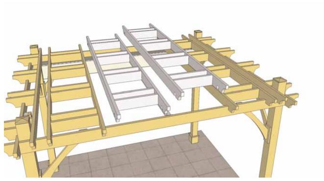
**1.** To make it easier to install Retractable Canopy Drive Beam, we recommend leaving center Ladder Sections off until Drive Beam and Canopy are attached.
