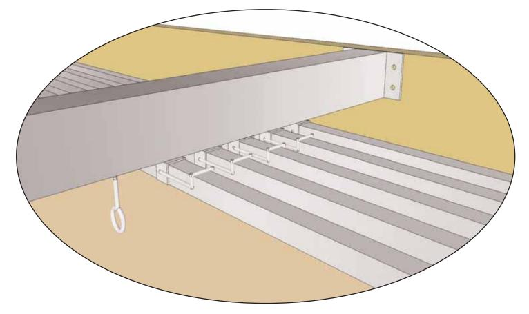
$\pmb{8}_{\:\raisebox{1pt}{\text{\circle*{1.5}}}}$  Complete remaining Canopy Locking Clip / Wing attachments.
