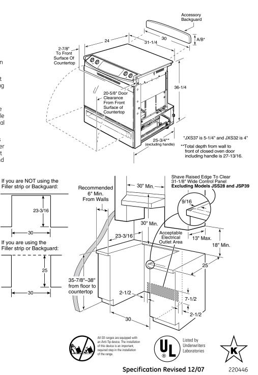
**Installation information:** Before installing, consult installation instructions packed with product for current dimensional data.
