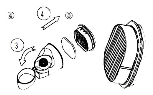
When the filters have been removed clean the filter chamber cones as well as any filters. Tapping filters on garbage can or blowing compressed air through filters can clean and extend the life of the filters.
