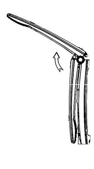
Step 4 - Put the electric floor brush tool on the floor as shown in the picture below; and then directly insert the floor brush and the upper part of the vacuum body together; at last press hard on the upper part of the vacuum body in a downward direction until you hear a "click" sound.
