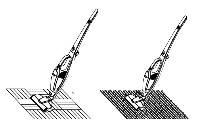
**SAFTEY FEATURE** – The Prolux Ion Stick Vac is a high end vacuum that is designed to last for years to come. As such it comes with an automatic brushroll shut off feature. If large debris (such as a sock) is sucked into the vacuum or string wraps around the brushroll the brushroll vacuum will automatically turn off. In this case make sure the unit is turned off, clear the obstruction from the brushroll, and turn the vacuum back on.
