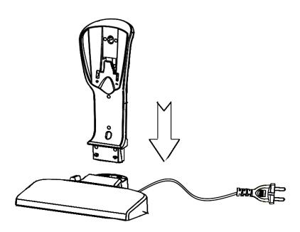
Step 2 – Assemble the charging dock station. As shown on the figure above, vertically insert front and rear cover of the charging dock component into the adaptor assembly until it is firmly connected together.
