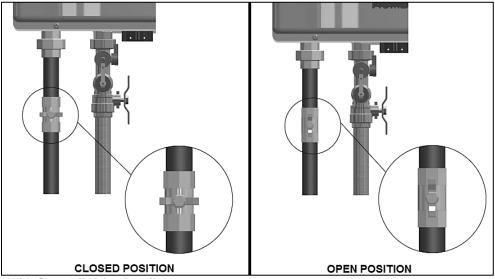
Figure 13 – Gas Line With Shut-Off Valve Detail
