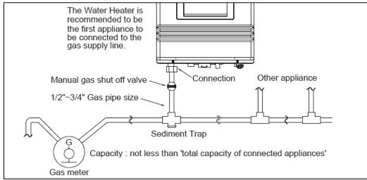
Figure 14 – Natural Gas Piping Installation – NOTE: Capacity to be not Less than Total Capacity of Connected Appliances
