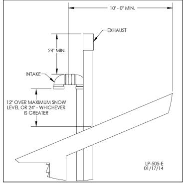
Figure 9 – Direct Vent, Vertical Termination
