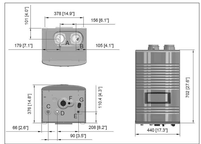
Figure 1 – Specifications and Dimensions
