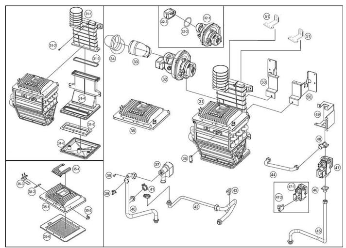
Figure 40 – Heat Exchanger Replacement Parts
