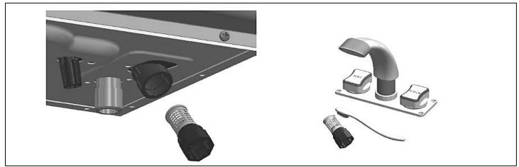
Figure 37 - Draining the Water Heater
