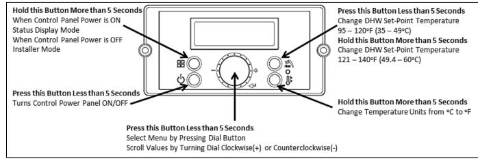
Figure 24 – Water heater Control Panel Detail
