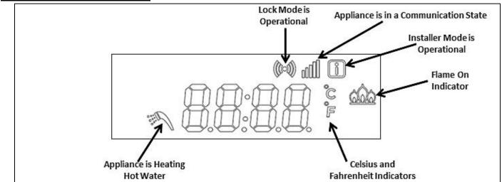
Figure 25 – LCD Display Detail
