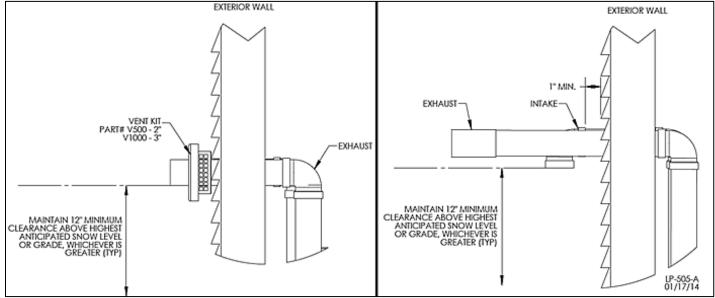
Figure 8 – Direct Vent, Sidewall Vent Termination
