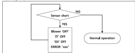
Figure 34 – Inlet / DHW / Operating Temperature Sensors Error Analysis Tree
