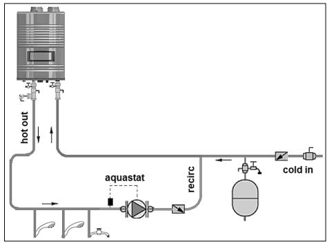
Figure 18 – Piping with Recirculation
