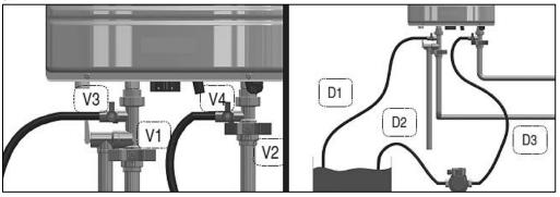
Figure 38 – Flushing the Water Heater
