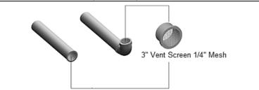
Figure 11 – Screen Installation - NOTE: Vent termination elbow is meant to be installed open end facing the ground. Orientation in Figure 11 is meant to demonstrate proper Vent Screen installation ONLY.
